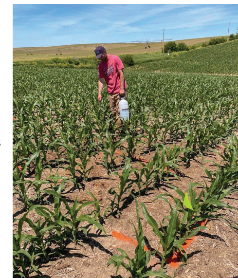
LLNRD technician Shay Reilly applies a bromide tracer to a test plot within a cornfield in Platte County.
