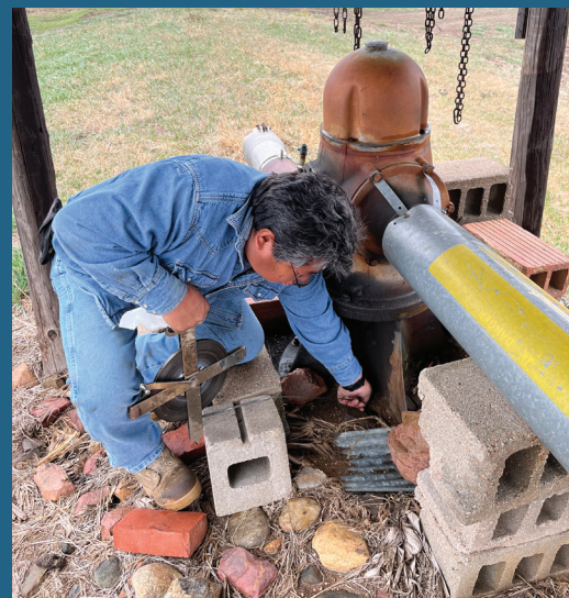
Below: Nemaha NRD Field Representative Tomas Chalé Aké measures water levels in the spring.
