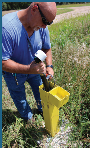
Below: Lower Niobrara NRD Water Resources Technician Gary Richardson launches telemetry into one of the district's monitoring wells.
