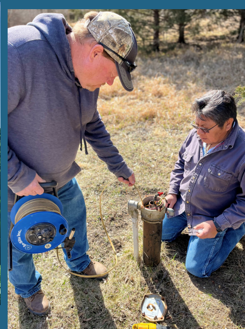
Nemaha NRD Field Representatives Mark McDonald, left, and Tomas Chalè Akè measure depth to groundwater this spring during a well blitz.
